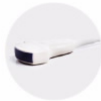
3.5MHz multi-frequency convex probe
